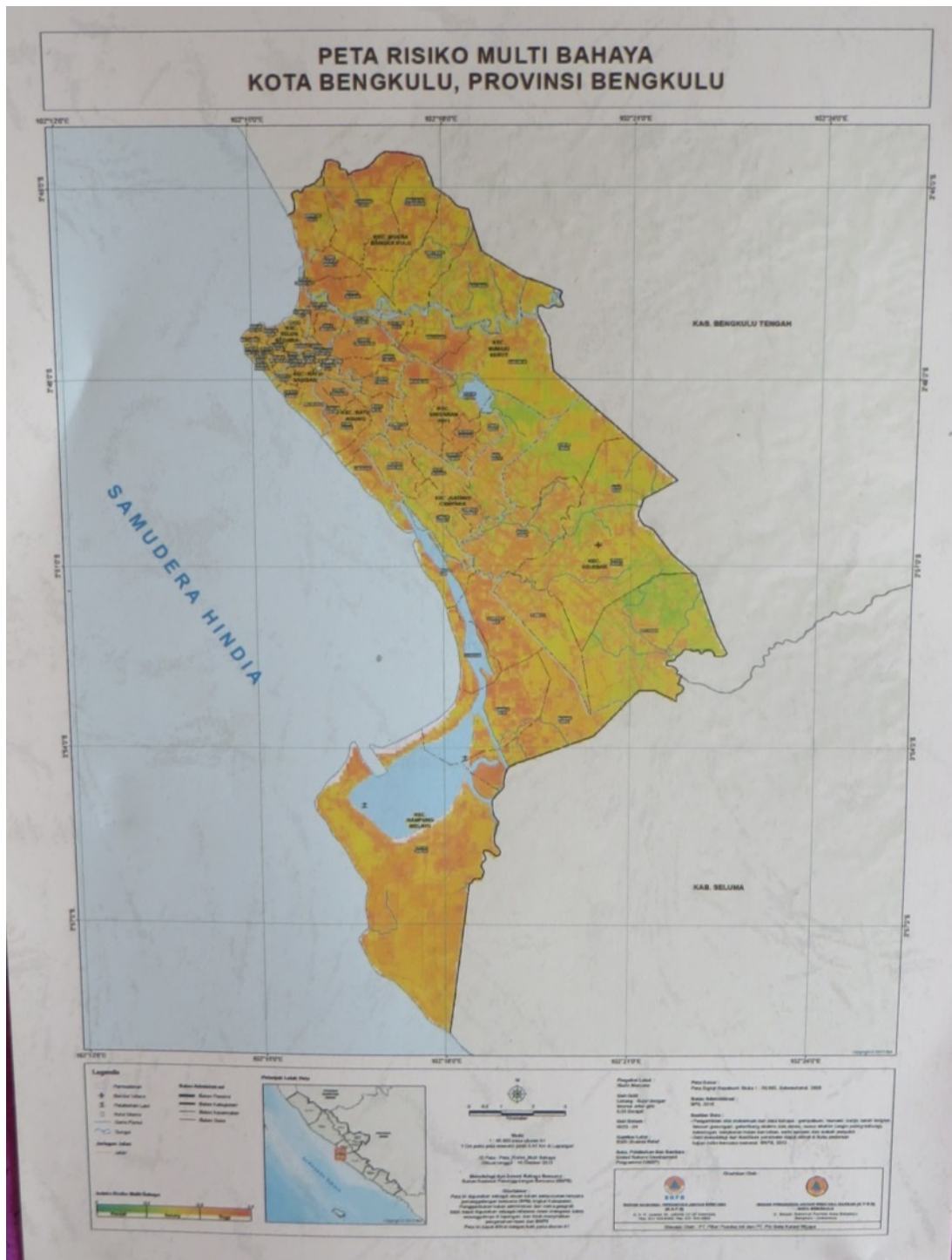
Figure 4: Multi-hazard Risk Map of Bengkulu City from BPBD Bengkulu City Office. Red and orange colours indicate higher risk and greens low risk
