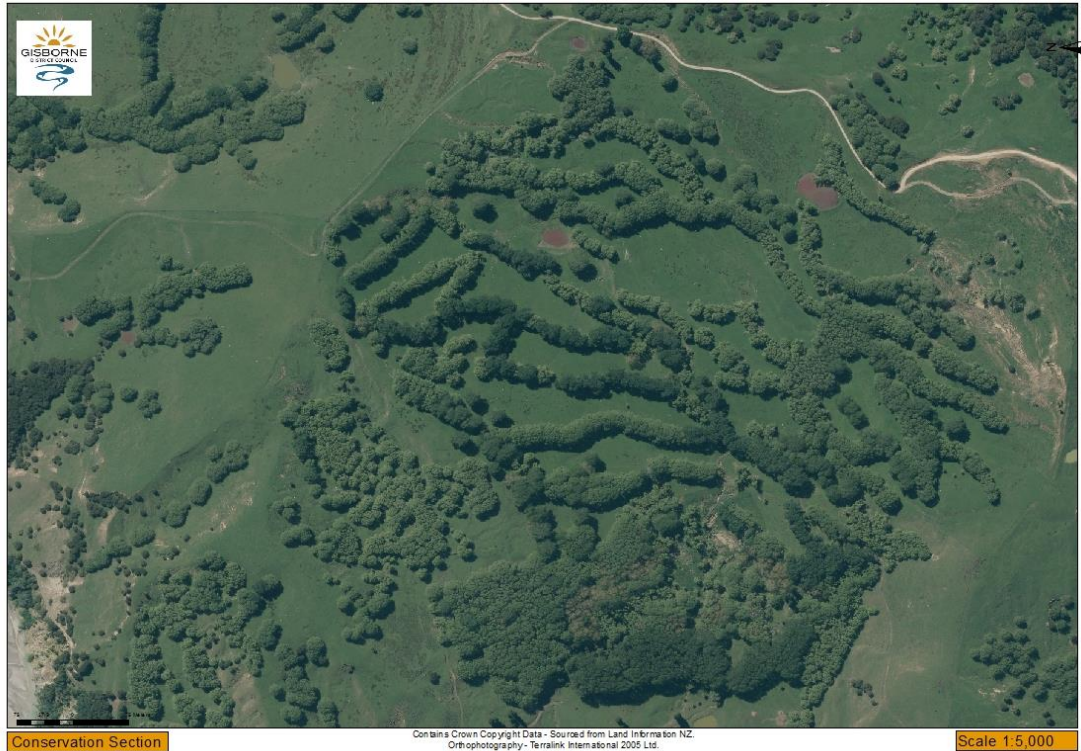
Figure 7 Poplar and Willow plantings supporting graded banks on earthflow erosion. Slopes were initially cultivated with graded banks constructed to direct runoff water.
