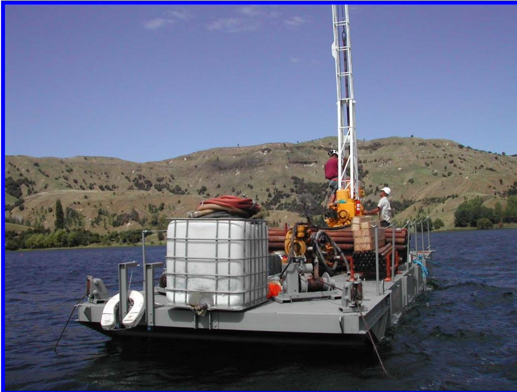
Figure 8 Drilling rig on Lake Tutira, used to obtain a 27m sediment core from the lake bed (~7000 year record)
