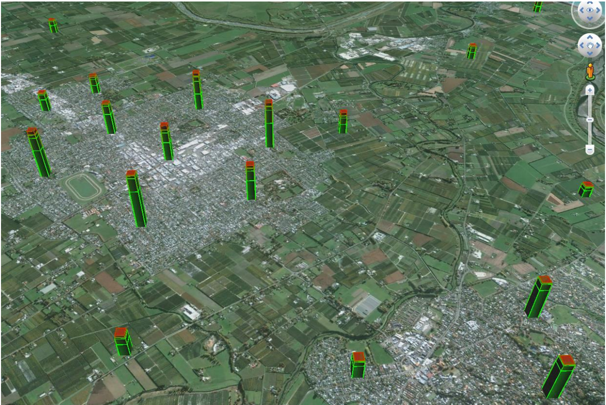
Figure 12 Damage distribution in Hastings District for earthquake generated shaking and associated liquefaction with a 500 year return period. The height of the stack indicates the number of buildings within the suburb and each colour band a different state of damage, the upper three being buildings unsafe to occupy and the lower stack being light or no damage.
