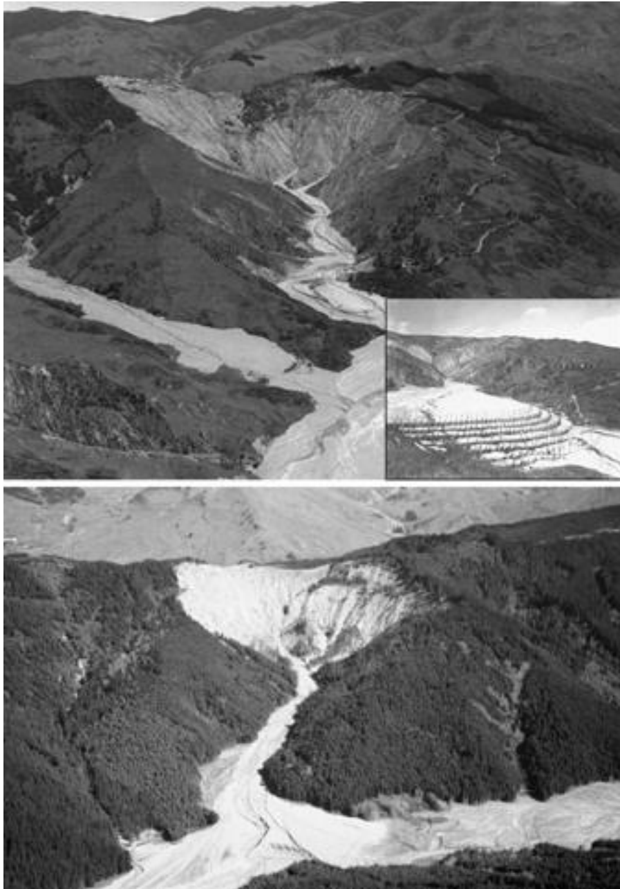
Figure 1 Tarndale Gully (pre-reforestation) with inset showing a fascine constructed with live poplar and willow materials in an attempt to retain sediment near its source, and post-reforestation with exotic pines (lower photo).
